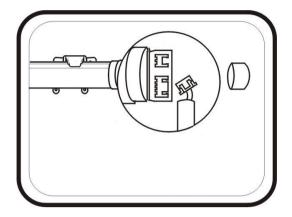
Another motor did not connect power supply; only connect 2 wires to 4pin.
